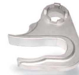
Aviation industry, Custom 465 Nitriding Depth: 18 μm ± 2 / 1100 HV
